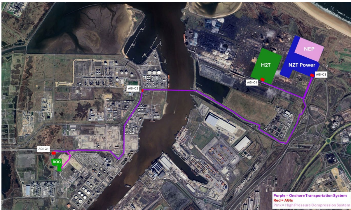
Figure 2: Teesside Onshore Transportation System map 1
